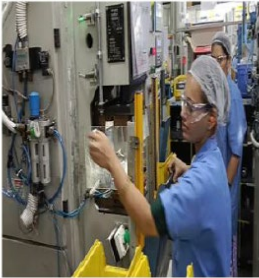
Fig.2 Relocating pressure gauge in arm's reach from working area
