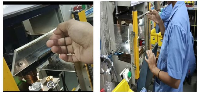
Fig.5 Obstructing Front Guard
